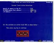
Gateway Communications' installation program simplifies the process of configuring the network interface card by using easy-to-follow diagrams (see screen shot above) to show you how to set the card's switches.
